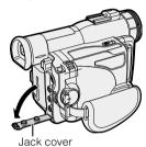
2 Connect the camcorder to your TV (or VCR) with the supplied audio/video cable, as shown.
